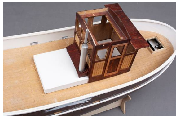
Fig. Position the superstructure on the hull
