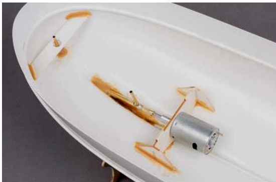
Fig. drive glued in hull
